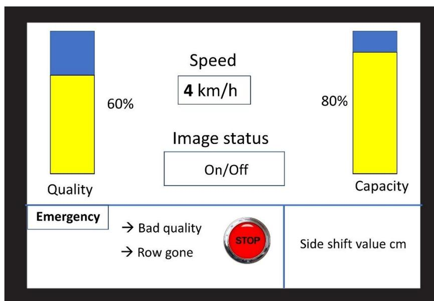
Figure 4. The ISOBUS mask for the weeder performance.
