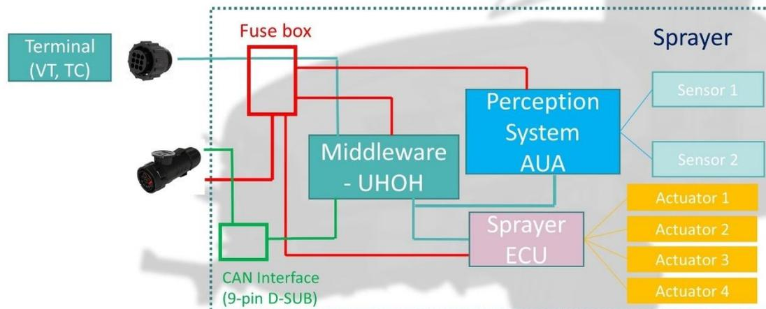
**Figure 1.** Schematic view of the smart sprayer.
