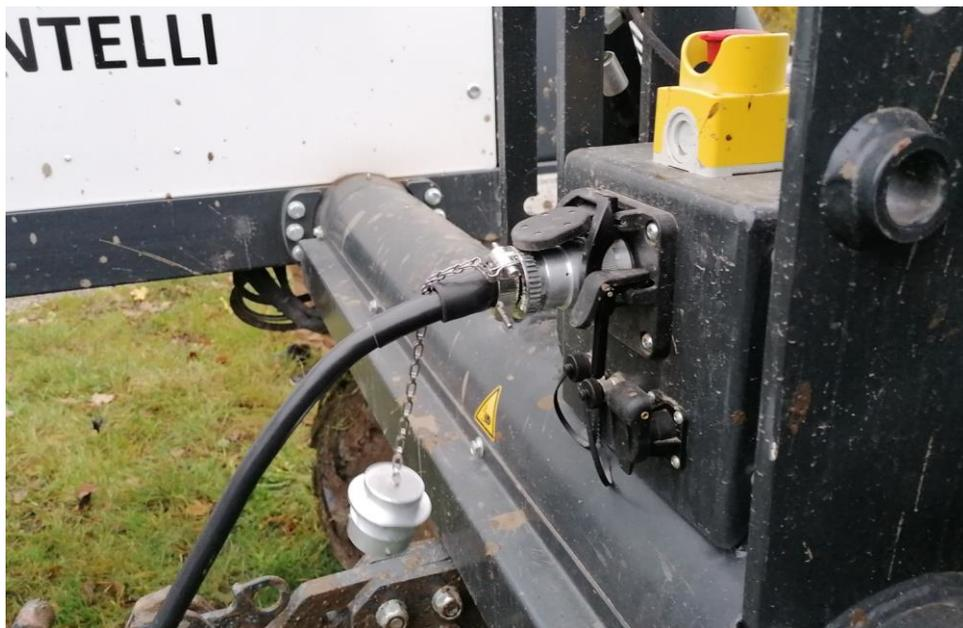
*Figure 22: Confirmed ISObus/power connection of middleware to robot*
