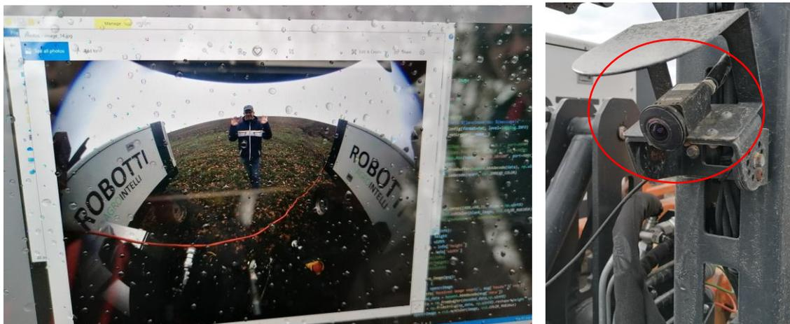
*Figure 19: Live image stream of Robotti cameras received by the analytics module (left picture) and camera hardware (right picture)*
