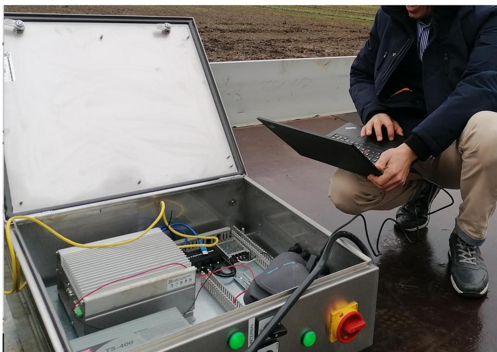
*Figure 20: Middleware PC placed inside electrical cabinet, connected and powered by Robotti via the thick, black cable in the foreground.*
