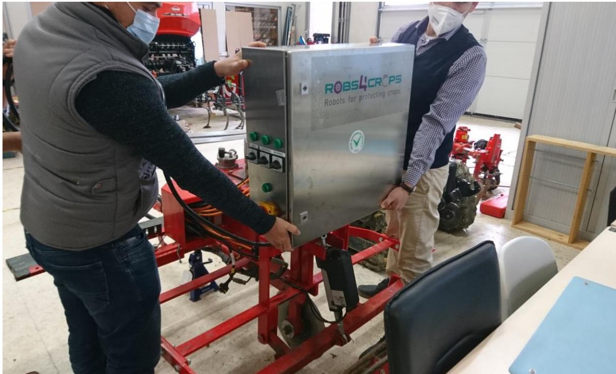
*Figure 2: Electric cabinet with middleware and analytics hardware mounted on implement*
