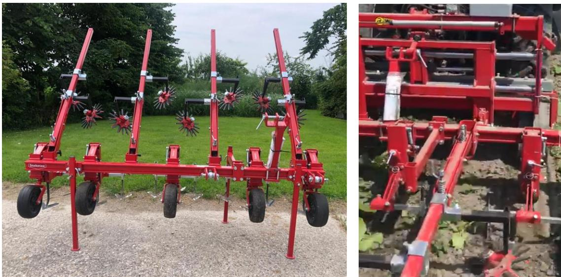
*Figure 18: Mechanical weeder implement used in LSP4 (left photo) and weeder implement together with the side shift module (right photo)*
