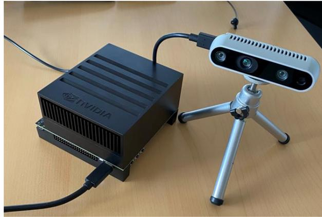
*Figure 13: Perception module consisting out of a NVIDIA Jetson embedded computer and Intel RealSense RGB-D camera.*
