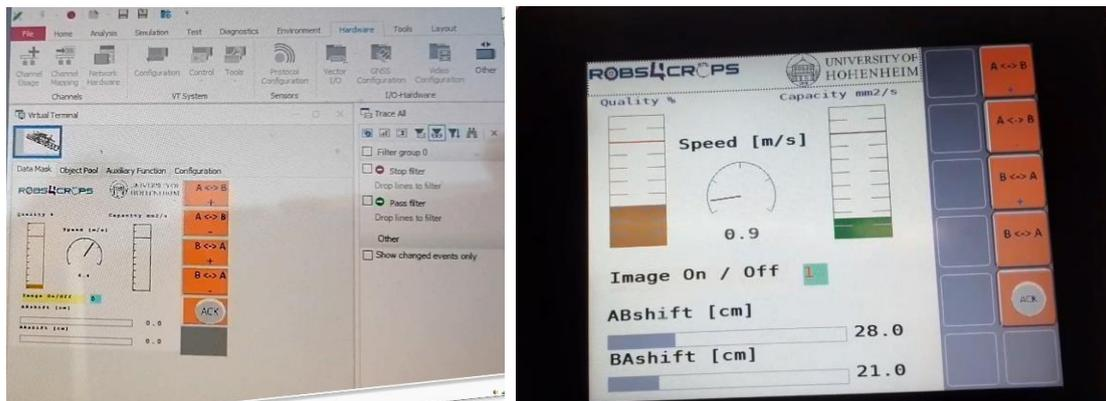
Figure 5: Virtual ISOBUS terminal showing information of the implement. Left image: software version of the virtual terminal in the middleware. Right image: photo of real virtual terminal hardware.
