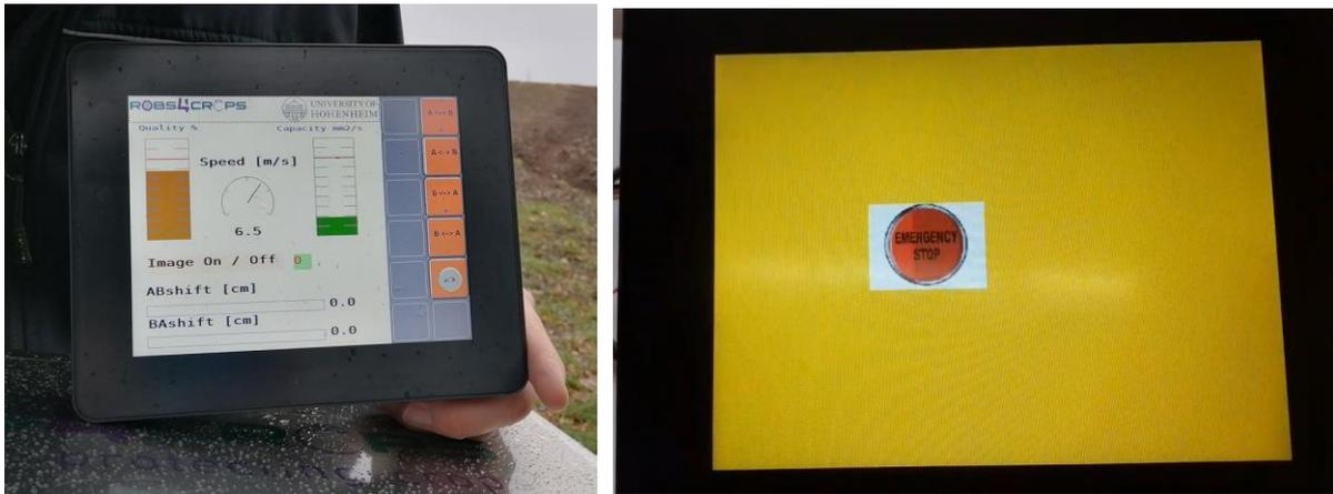
Figure 25: ISObus terminal showing live status information of the Robotti and of the analytics module (left photo: status information, right photo: emergency stop message)
