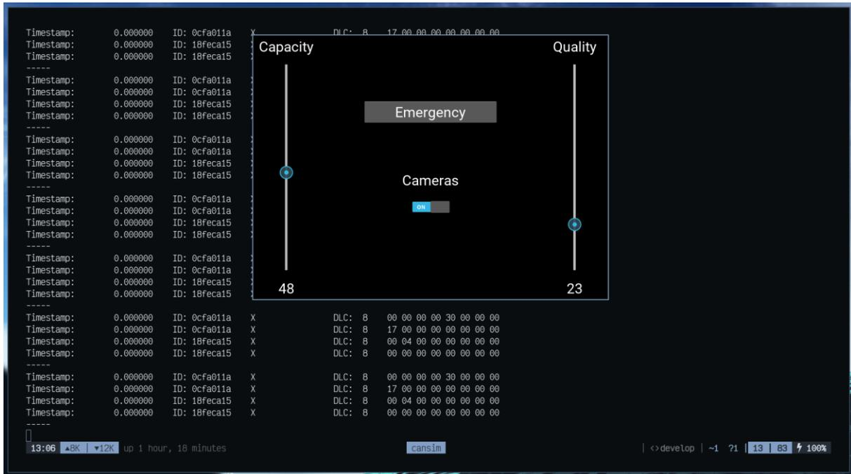
Figure 4: Screenshot of “ANALYTICS SIMULATOR” sending CAN messages to the middleware. The window in the centre of the screen has controls that can be used to simulate messages that the weeding implement sends to the vehicle.
