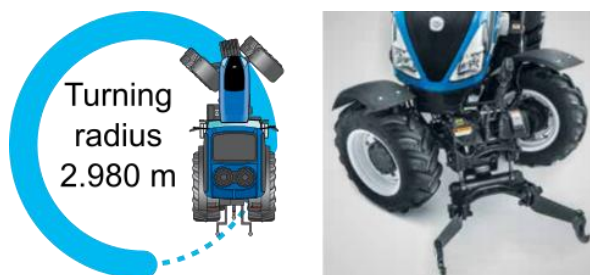
Figure 20. Turning radius for the retrofitted tractor T4.F100.
