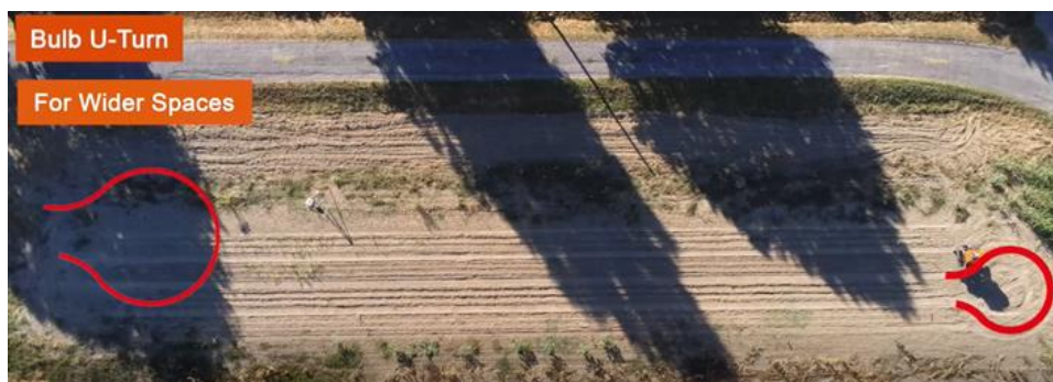
Figure 19. Bulb U-turn for the CEOL robot.
