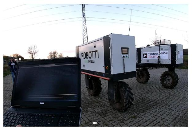
Figure 27: Starting and stopping real Robotti by commands from the FC
