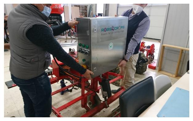
Figure 2: Electric cabinet with middleware and analytics hardware mounted on implement
