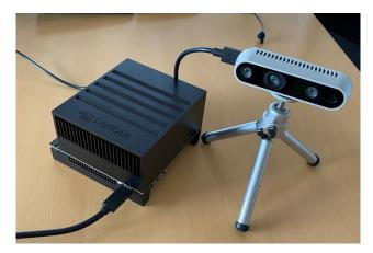
Figure 13: Perception module consisting out of a NVIDA Jetson embedded computer and Intel RealSense RGB-D camera.
