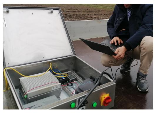
Figure 20: Middleware PC placed inside electrical cabinet, connected and powered by Robotti via the thick, black cable in the foreground.
