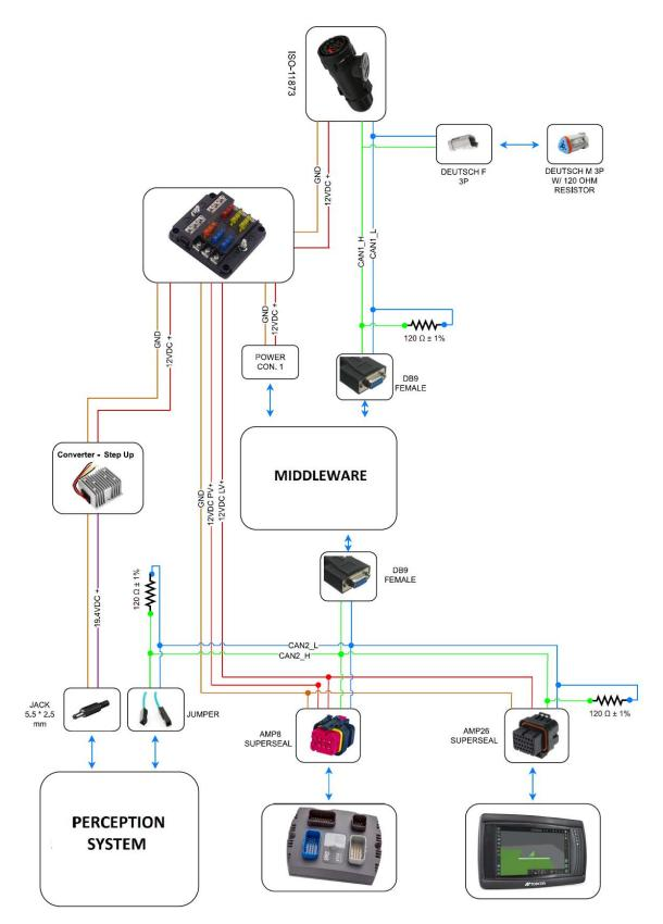
Figure 12: Schematics of the sprayer cable harness including the ECU of the sprayer, the crop perception system and the middleware
