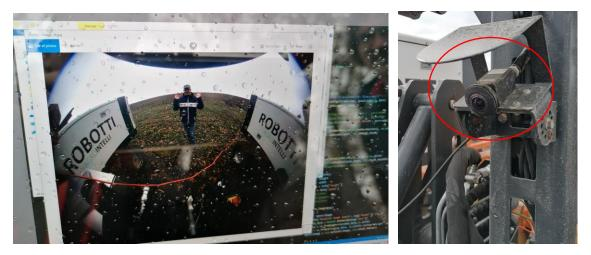
*Figure 19: Live image stream of Robotti cameras received by the analytics module (left picture) and camera hardware (right picture)*
