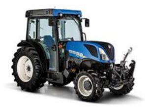
Figure 17: New Holland T4-100F, narrow width orchard tractor (to be retrofitted for MVP2 and MVP3)
