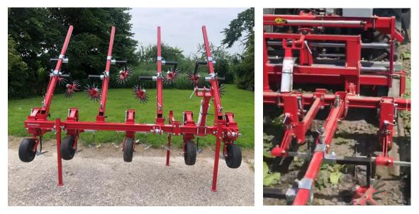
Figure 18: Mechanical weeder implement used in LSP4 (left photo) and weeder implement together with the side shift module (right photo)
