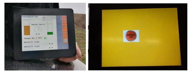
Figure 25: ISObus terminal showing live status information of the Robotti and of the analytics module (left photo: status information, right photo: emergency stop message)
