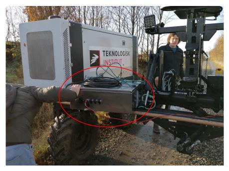
Figure 21: Electrical cabinet/Fuse box (encircled) connected to Robotti
