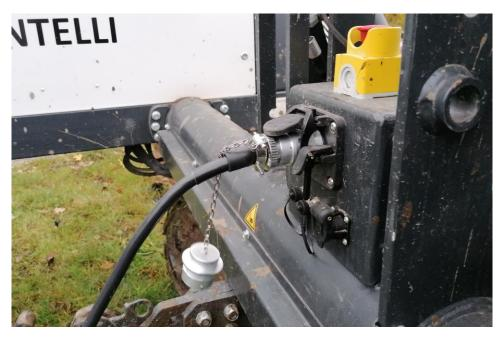
Figure 22: Confirmed ISObus/power connection of middleware to robot
