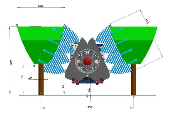
Figure 10: Illustration of the working principle of the ASM 200 sprayer of Teyme in the vineyard
