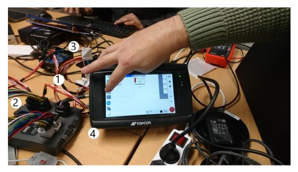
Figure 11: ISOBUS virtual terminal showing status information. 1 – Physical harness of the sprayer (Prototype version, but completely functional), 2- Sprayer ECU 3- Crop Perception module, 4-ISOBUS virtual terminal
