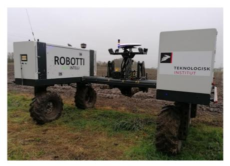
Figure 23: Robotti as autonomous vehicle
