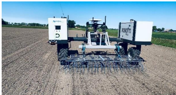
Figure 8: Tine weeding in pumpkins with Robotti
