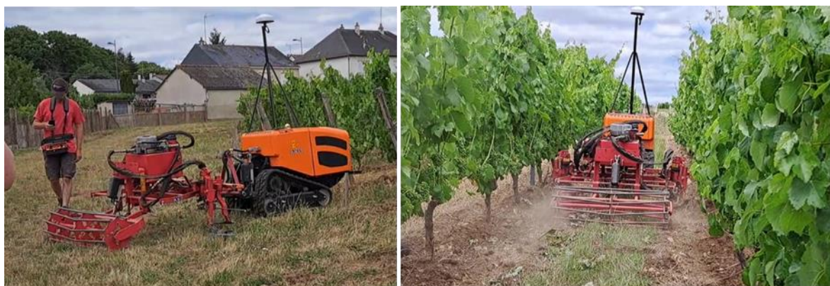
Figure 1: CEOL robot with a mechanical weeder implement as used in the LSP1 in 2022
