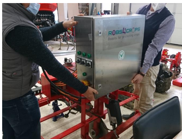
Figure 4: Bulky electronics cabinet with middleware and analytics hardware mounted on implement
