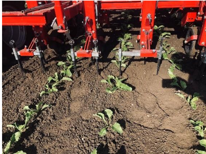
Figure 12: One hoe is in the row, destroying the beets because of side-shift problem
