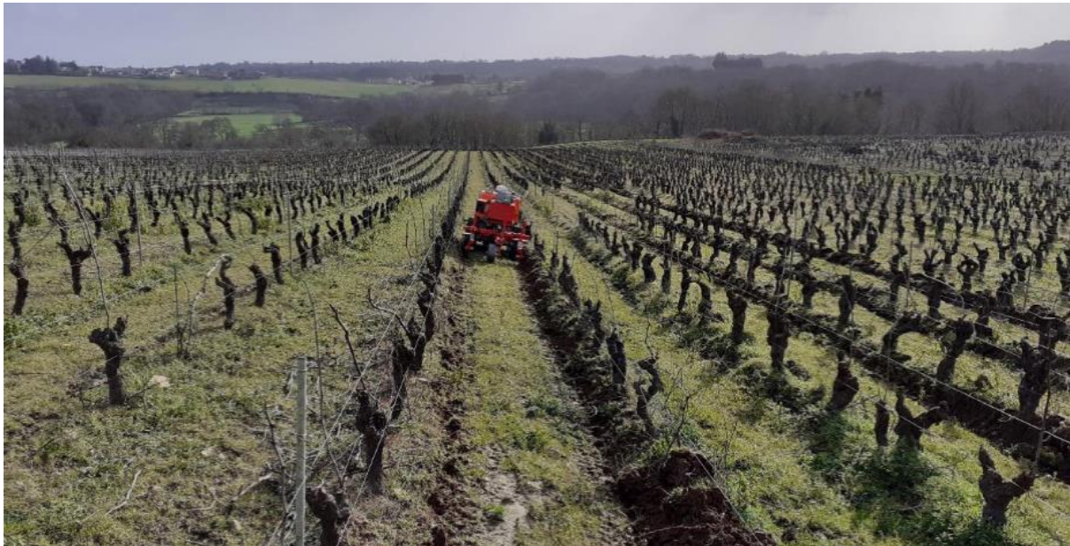
Figure 3: Slope, the CEOL has trouble staying on track
