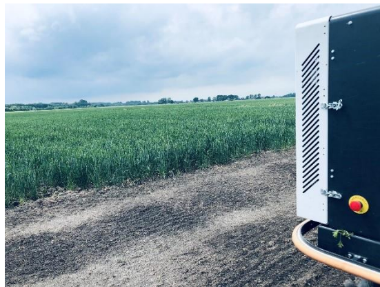
Figure 10: Barley field next to pumpkin field frequently activated the Robotti's LIDAR sensor-based emergency stop.
