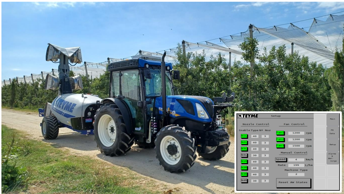
Figure 7: MVP1 in the LSP3 with New Holland T4 110F Tier 4B tractor and the TEYME EOLO 2000 sprayer and on the bottom right a screenshot of the TEYME sprayer interface.
